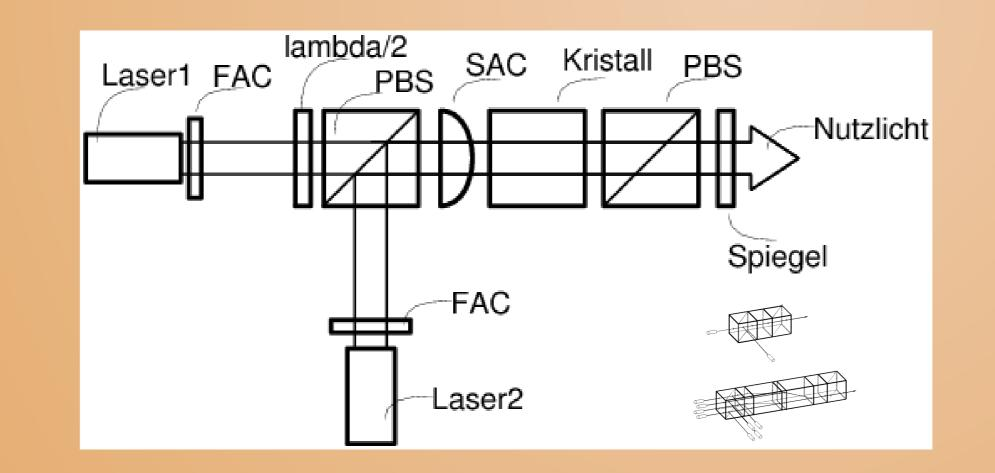
Two (semiconductor) laser are polarization coupled. The combination of a birefringent crystal between two polarizers operates as a narrow bandwidth Lyotfilter. The laser lines lock to their respective wavelengths by means of a feedback-mirror. Due to the polarization beamsplitter the two laser emissions are orthogonal on the side of the semiconductors and parallel on the side of the outcoupling mirror.
